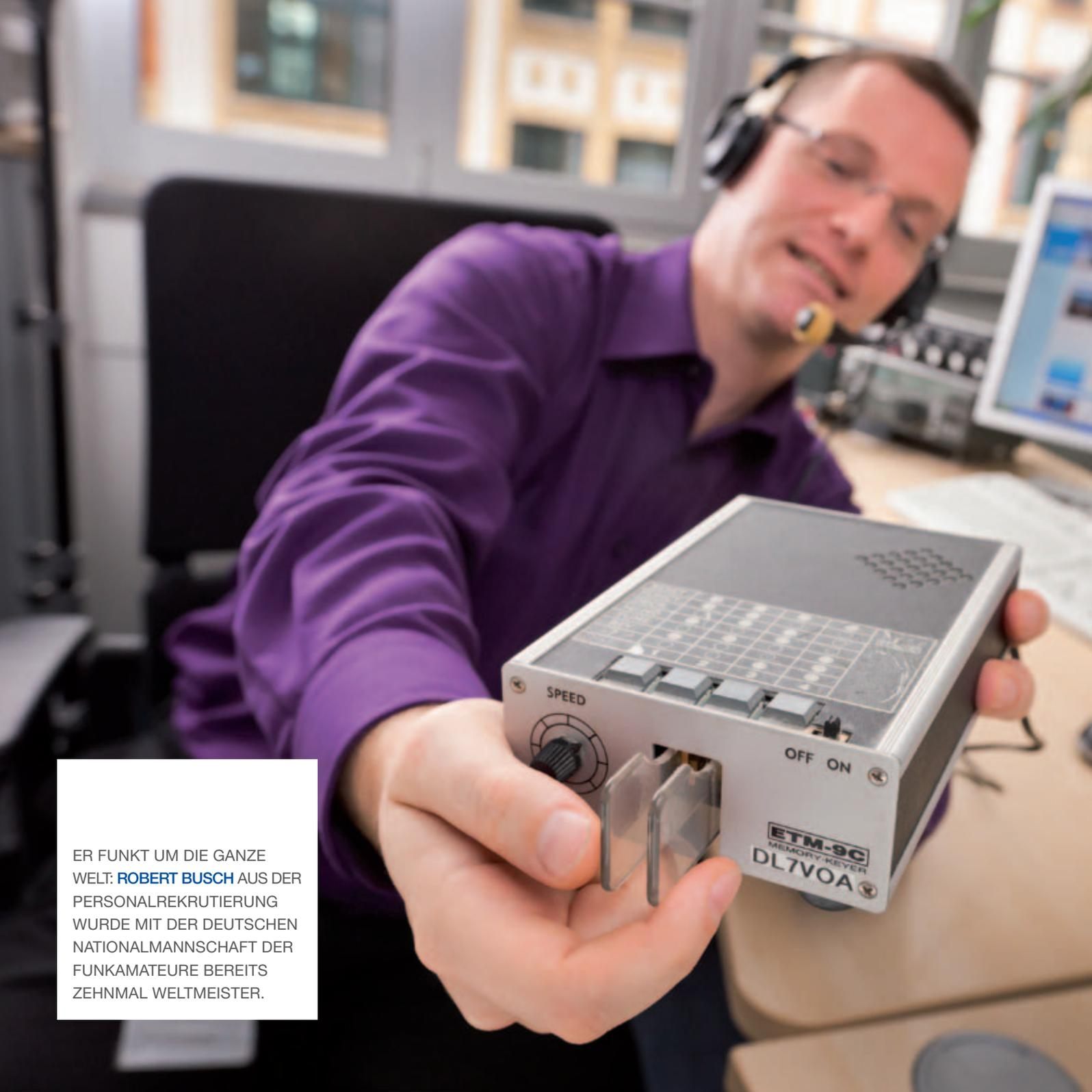
A man wearing a purple long-sleeved shirt and a headset is sitting at a desk in an office. He is holding a silver electronic device, a memory keyer, in front of him. The device has a grid of buttons on top, a speaker, and a control knob labeled 'SPEED'. The brand name 'ETM-9C MEMORY-KEYER DLTVOA' is printed on the front. The background shows a computer monitor and office equipment.
